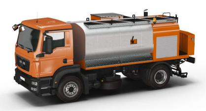
Strassmayr Gold emulsion sprayer is designed for high precision emulsion spraying on big surfaces. Gold equipment line ensure comfort and easy control of all machine functions automatically. Speed addicted spraying and fully automated cleaning installation makes each spraying job quick, precise and easy. Operator has full control of machine functions on the touch panel in the truck cabin.
