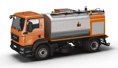
Strassmayr Platinum emulsion sprayers are the most technologically advanced from the entire line-up. Machine's purpose is to spray the surface with the highest precision and effectiveness. The operator is able to control the unit directly from the driver's cabin on the large touch screen covering all the functions of the machine. Fully automatic cleaning installation and speed addicted spraying make TS Platinum the most high-tech solution in road building industry.
