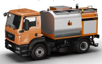
Strassmayr Silver emulsion sprayers are created for evenly and effective spraying the roads with emulsion. Equipped with special elliptic tank covered by aluminum, automatic computer control of spraying and manual valves for emulsion circuit, ensures highest quality of spraying for reasonable price. Computer control ensures the maintaining of constant pressure of sprinkling emulsion even by changing speed or spraying width.
