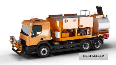
The **STRASSMAYR STP 1010** Blow Patcher allows reparation of holes and damages in the road surface without using the milling machine and paver, on behalf of emulsion and aggregates. This type of machine requires only two man to operate and fulfill the technology of road surface repairs (the operator and the driver of a truck). Machine is equipped with the most modern material delivery systems, including electronic control over the mixing process.
